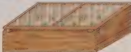
A cold frame consists of a wood or metal framework fitted with glass or rigid plastic panels.
