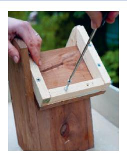
Measure and cut four wooden batons from the sawn timber to fit along the front and back edges of the birdhouse roof, angling one end of each of them so that they marry up at the top. Pre-drill holes in the wood and screw the wooden batons onto the roof. Measure and cut another two batons to fit along the side edges of the roof, pre-drilling and screwing them between the front and back pieces, as shown.
