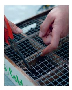
Using the wire cutters or scissors, cut a vertical hole in the mesh and then make a small line of cuts at the top and bottom of the first one in order to create two flaps that you can open out a little.
