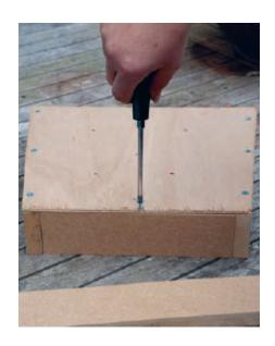
Again, using the pre-drilled holes as a guide, screw the front and back batons into position between the side batons to make a sturdy box. Finally, screw the piece of hardboard in place along the front and back edges.
