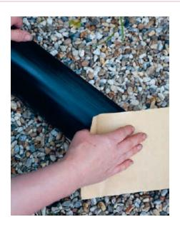
Using the hacksaw, cut two lengths of guttering, about 30in (75cm) in length. Rub sandpaper all over the guttering, end pieces, and brackets to make the surfaces rough so that the paint will adhere well.
